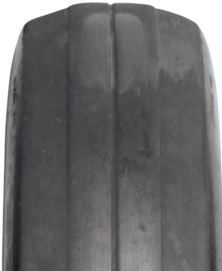
Figure 507. Shoulder Wear due to Underinflation
