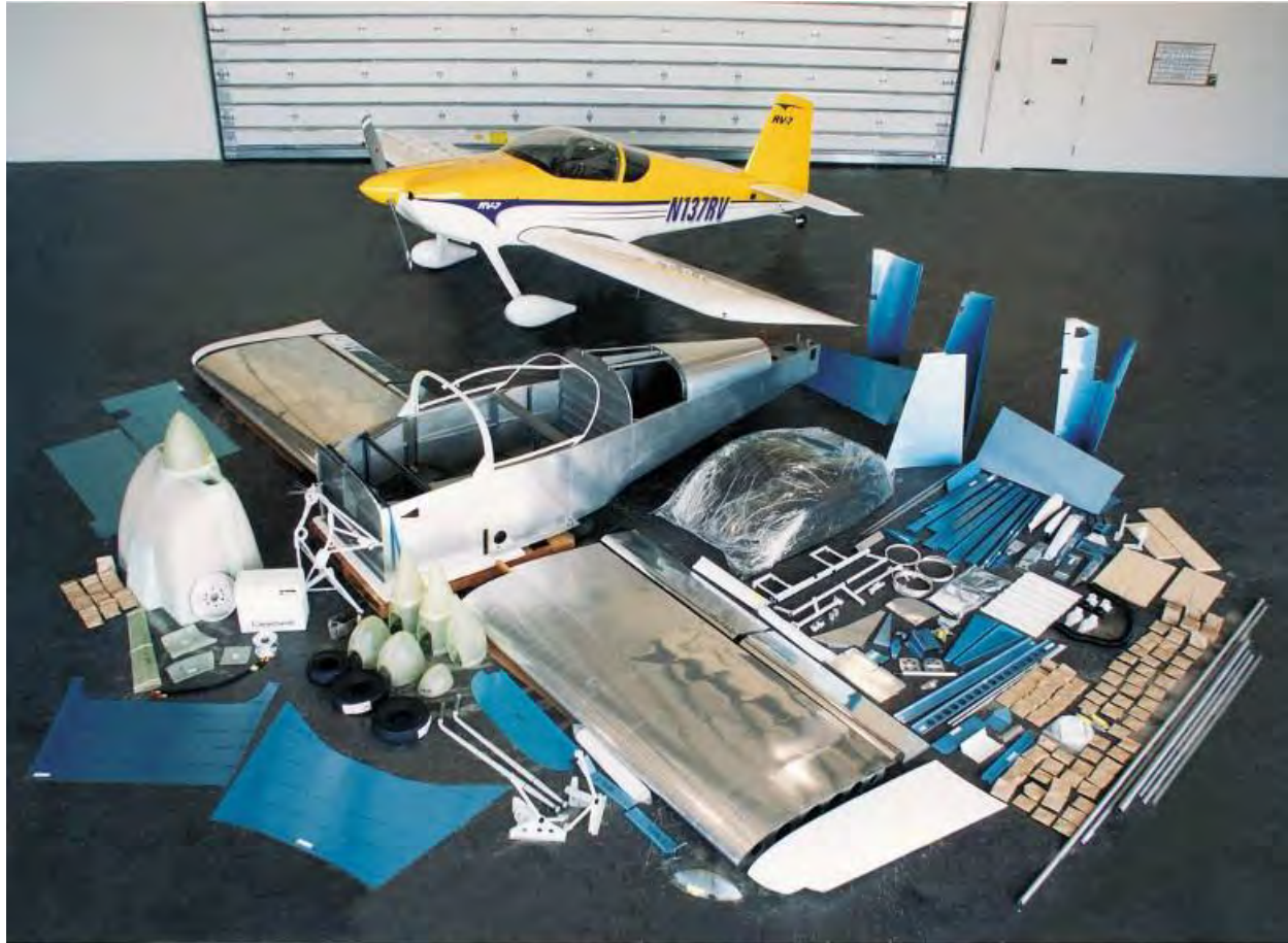
Figure 4. The quick-build kit of Van's RV-7 airplane.
