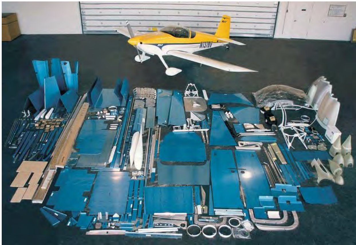
Figure 3. The standard build kit for Van's RV-7 airplane.
