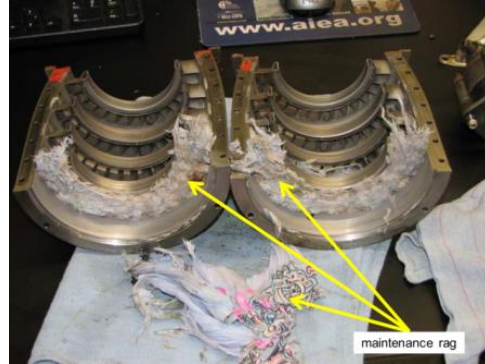
Figure 4. Compressor case halves removed.
