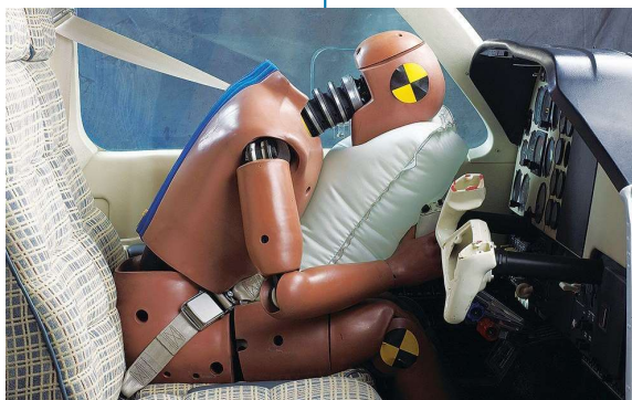
AmSafe's Seatbelt Airbag System (SOARS) is an example of an aftermarket lapbelt airbag restraint system, which is designed to mitigate head and torso injury in aircraft crash conditions. Photo courtesy AmSafe, Inc.
