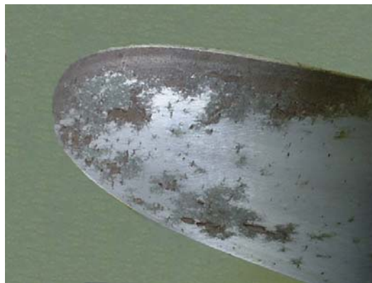
FIGURE 1-2. Polished Blade Surface Corrosion
