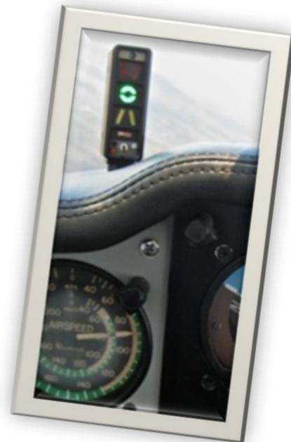
An AOA indicator can be used to get the pilot's attention (via audio and/or low cost stick shakers) even if the pilot is not looking at it. This focuses the pilot's attention on where it needs to be to avoid the stall. It can also help when used in conjunction with airspeed and existing stall warning systems, when available.
