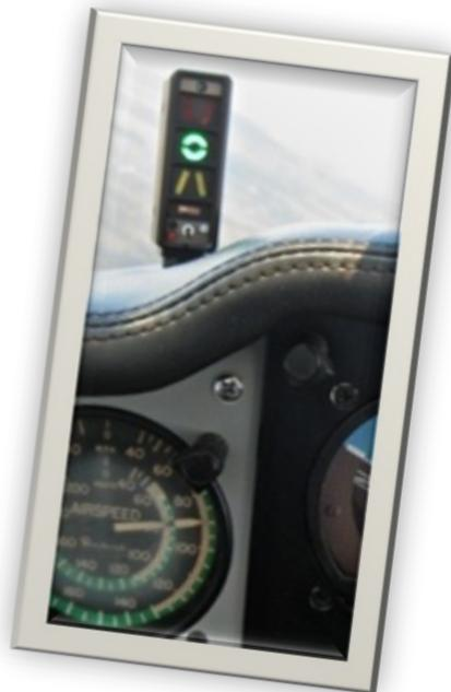
An AOA indicator can be used to get the pilot's attention (via audio and/or low cost stick shakers) even if the pilot is not looking at it. This focuses the pilot's attention on where it needs to be to avoid the stall. It can also help when used in conjunction with airspeed and existing stall warning systems, when available.
