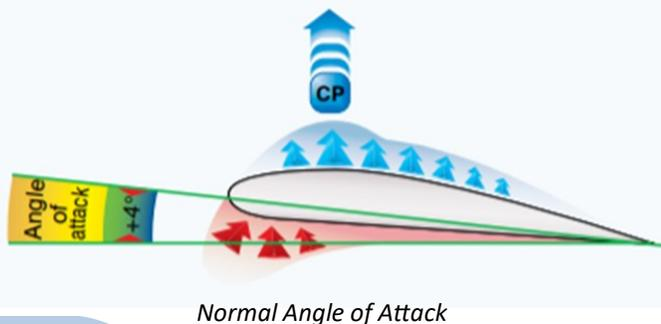
stall speed (as do other factors such as gross weight, center of gravity, and flap setting). Therefore, it is possible to stall the wing at any airspeed, at any flight attitude, and at any power setting.
