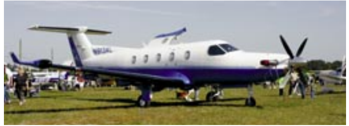
Pilatus PC-12 executive/corporate Turboprop can seat up to nine passengers in comfort and cruise at 280 kts with 1,500 nm range. It can readily operate out of Simsbury Airport as it did at the 2008 Fly-In, above.
