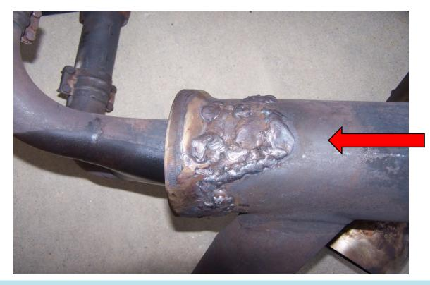
Improper weld per AC43.13 1B
