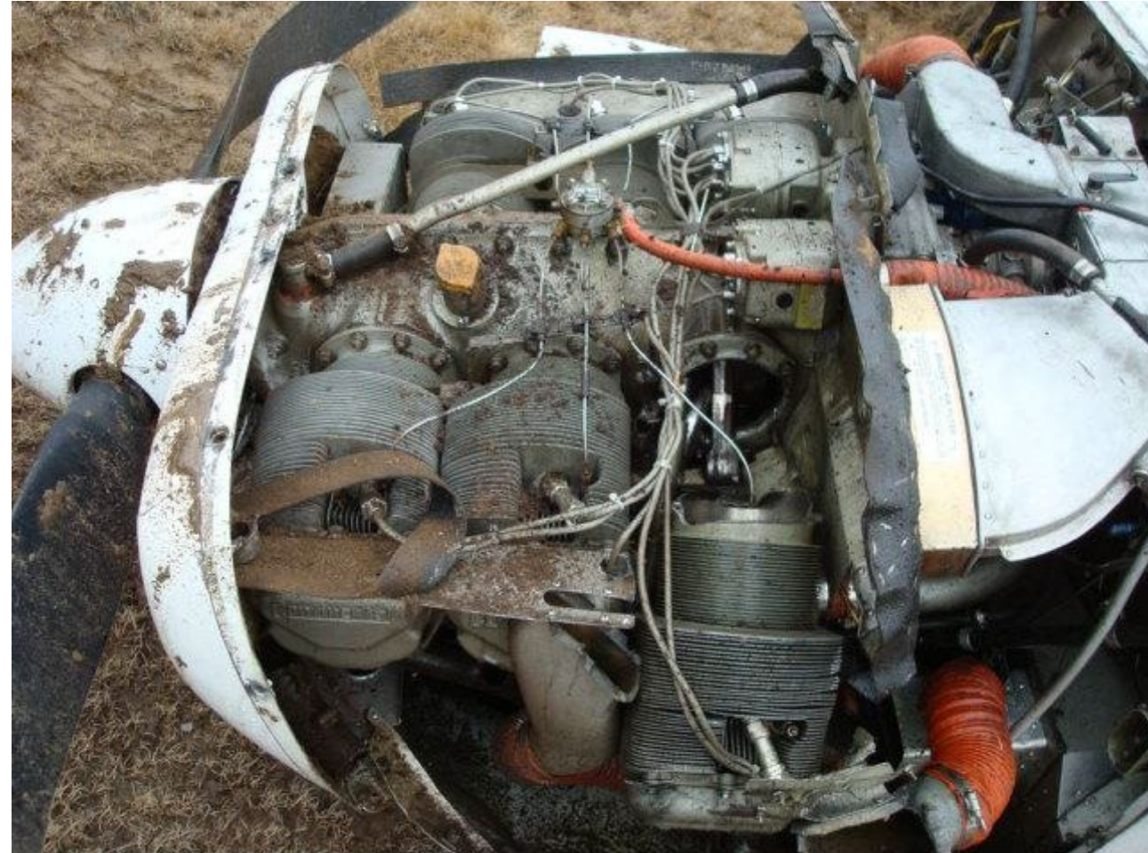
Photo 2. The engine after cowling removal. Note separated number 2 cylinder.
