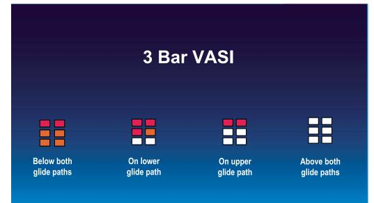
Three Bar VASI installations provide two visual glide paths. The higher glide path is intended for use only by high cockpit aircraft (Boeing 747, DC10) to provide a sufficient threshold crossing height.
