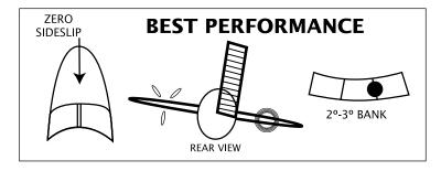
Figure 3. Asymetrical thrust counteracted by both rudder and aileron input.
