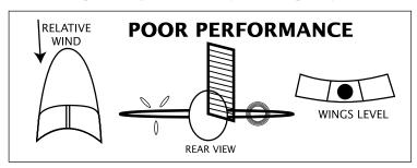
Figure 1. The result of rudder-only correction.
